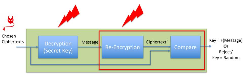
Modus Operandi: Inject Faults to realize a Decryption Failure (DF) Oracle
