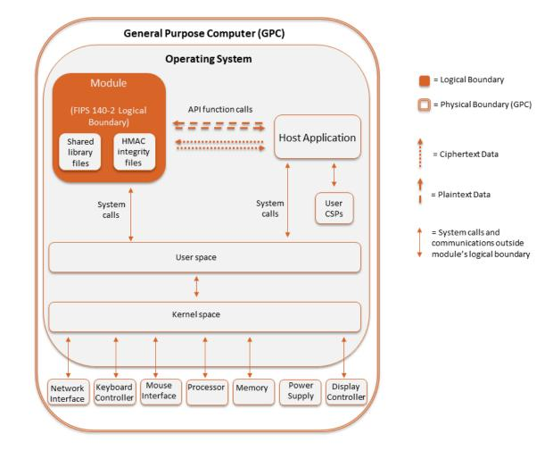
The figure below shows the module's physical and logical block diagram:
