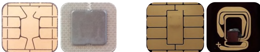
Figure 1 – Contact only: P-M4.8-8-1 front and back (left); S-MFC6.8 front and back (right)
