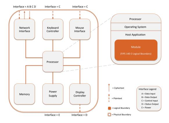
Figure 1 – Module Boundary and Interfaces Diagram
