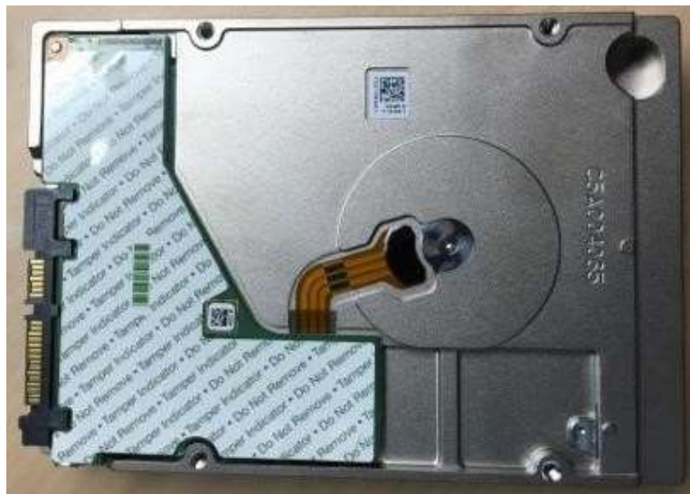
Figure 1: Tamper-Evident Security Label on PCBA to Provide Evidence of PCBA Tampering
