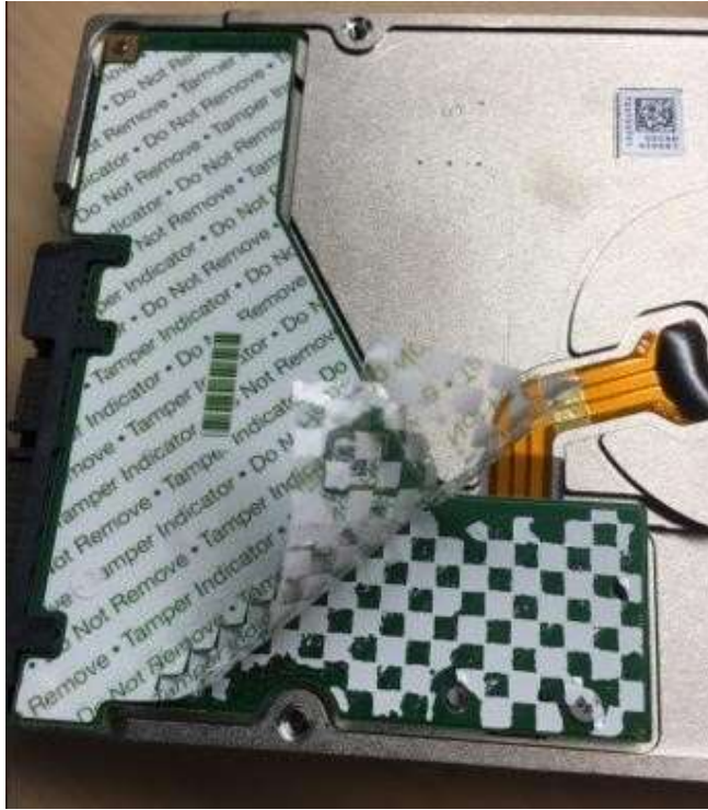
Figure 2: Tamper Evident Security Label on PCBA Showing Evidence of Tampering
