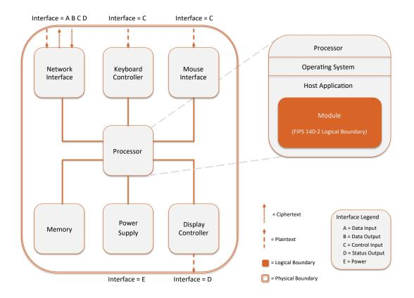
Figure 1 – Module Boundary and Interfaces Diagram
