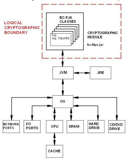
Figure 1 - Block Diagram of the Software for the BC-FJA Module.
