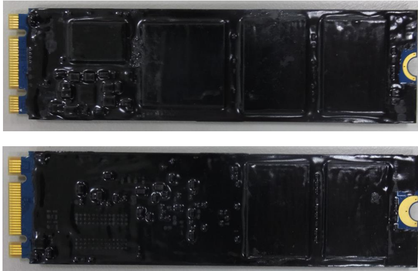
Exhibit 3 - Specification of the PS3112-S12 M.2 2280 SATA NAND FLASH SSD (D3) Series Cryptographic Boundary (From top to bottom: top side, bottom side).
