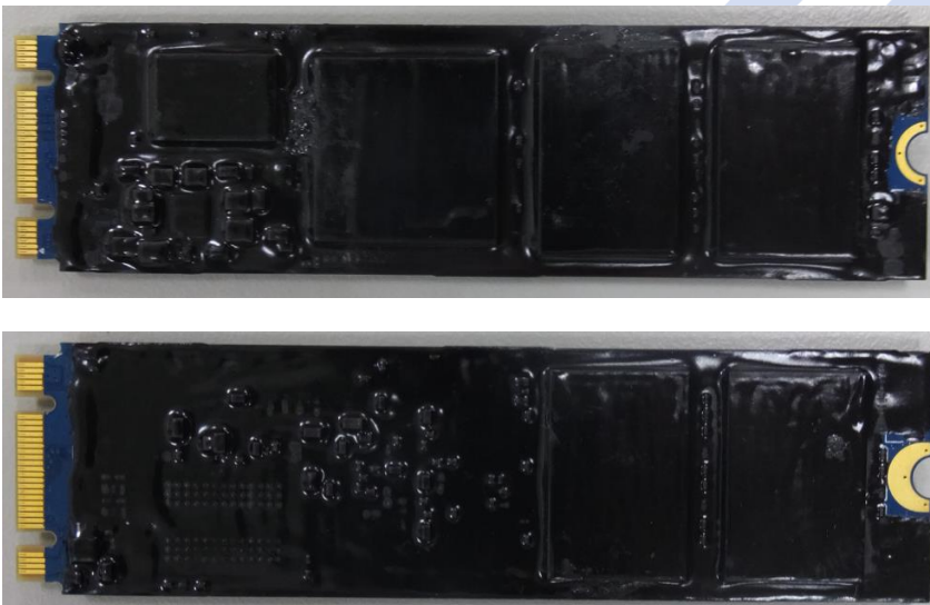
Exhibit 3 - Specification of the M.2 2280 SATA NAND Flash SSD Cryptographic Boundary (From top to bottom: top side, bottom side).
