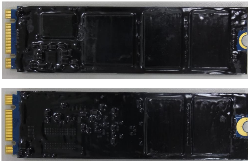
Exhibit 3 - Specification of the KSED300-S M.2 2280 SATA NAND FLASH SSD Series Cryptographic Boundary (From top to bottom: top side, bottom side).
