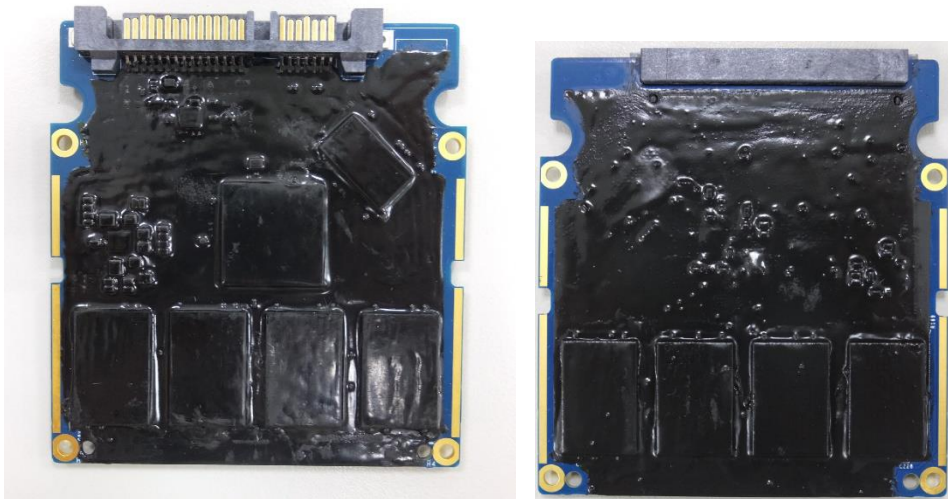
Exhibit 2 - Specification of the KSED300-S 2.5-INCH SATA NAND FLASH SSD Series Cryptographic Boundary (From left to right: top side, bottom side).
