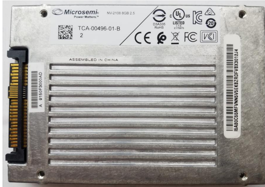
Figure 2 – Microchip NV-2108 (Bottom View)
