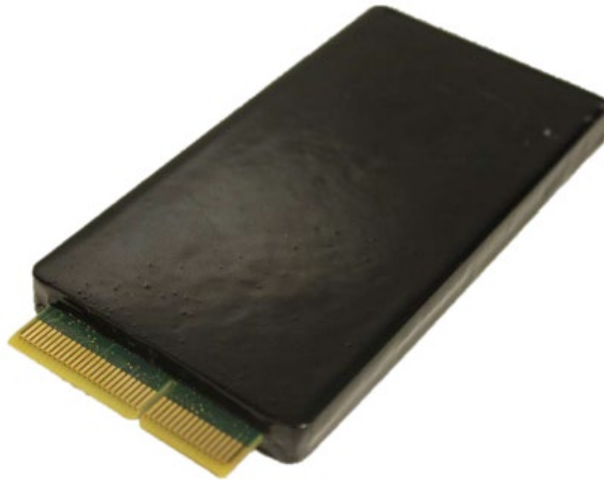
Figure 2 – EXP1000 with its Tamper Potting Intact
