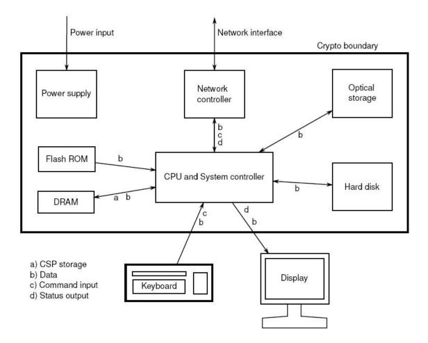
Figure 2 - Cryptographic Module Physical Boundary
