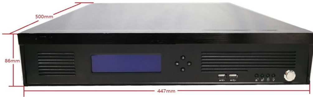
Figure 2 – The Sansec HSM device and its physical external dimensions
