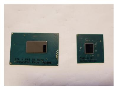
Figure 1b – Intel Cannon Point PCH with Coffee Lake (CFL) chipset
