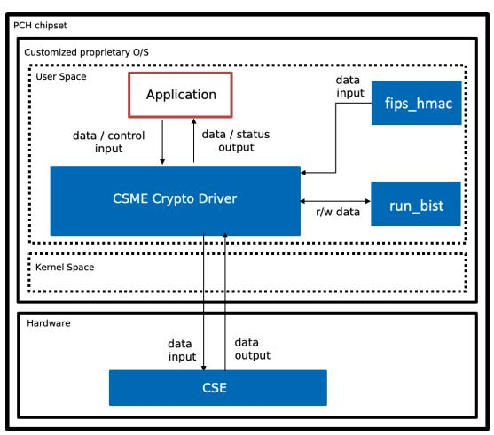
Figure 2 - Logical Block Diagram
