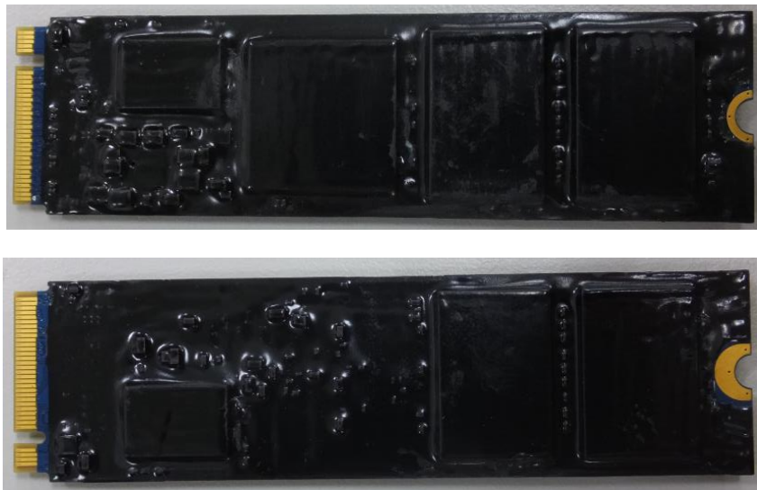
Exhibit 2 - Specification of the Cigent Secure SSD Advanced FIPS M.2 2280 Cryptographic Boundary (From top to bottom: top side, bottom side).
