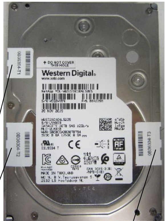
Figure 5: Wrapping Tamper-Evident Seals
