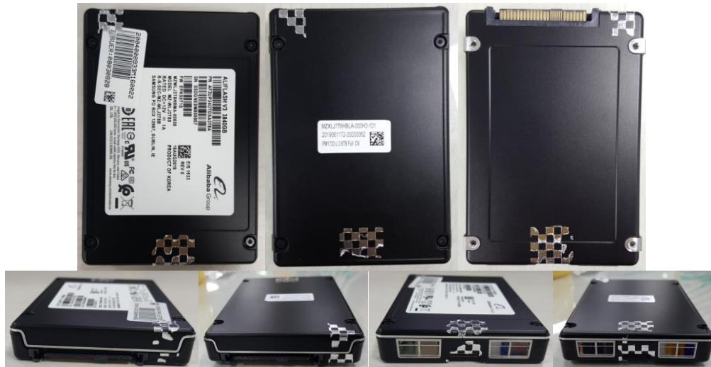
Exhibit 16 – Example of Signs of Tamper
