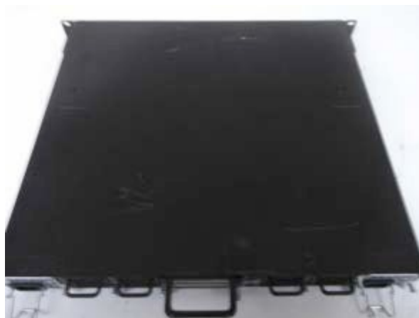
Figure 20 - Bottom side of the ICX 7750-48F
