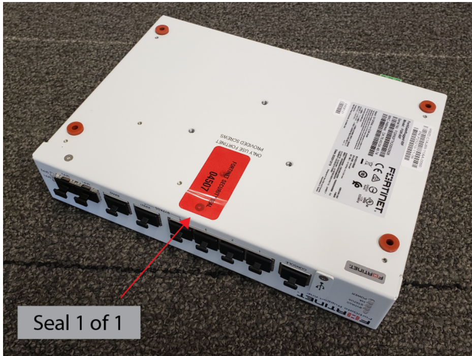
Figure 20 - FortiGateRugged-60F external enclosure seal, bottom
