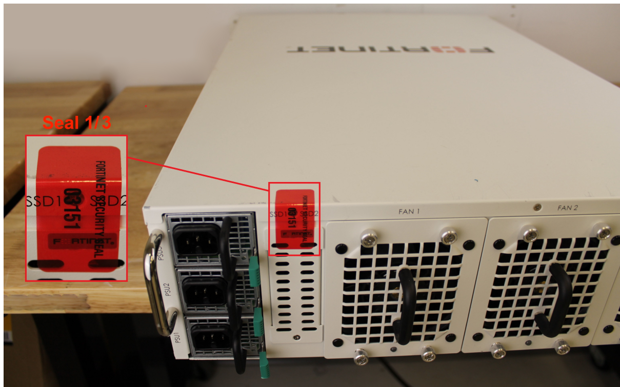
Figure 37 - FortiGate-6300F/6301F/6500F/6501F external enclosure seal 1, top, rear
