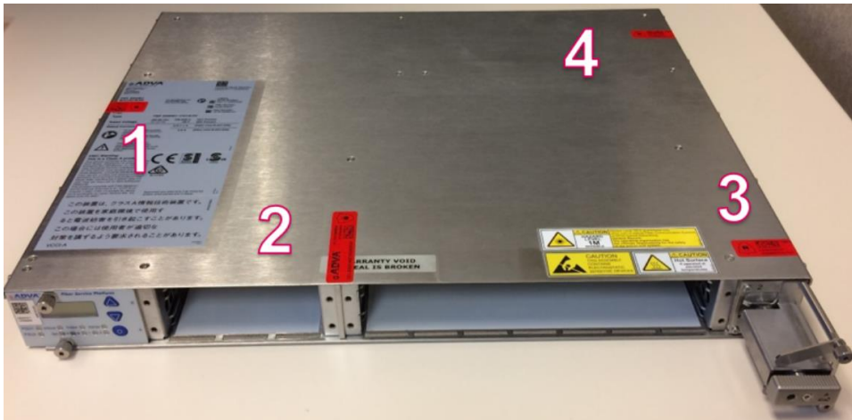
Figure 26: Placement of seals SH1HU-R/PF front-top view
