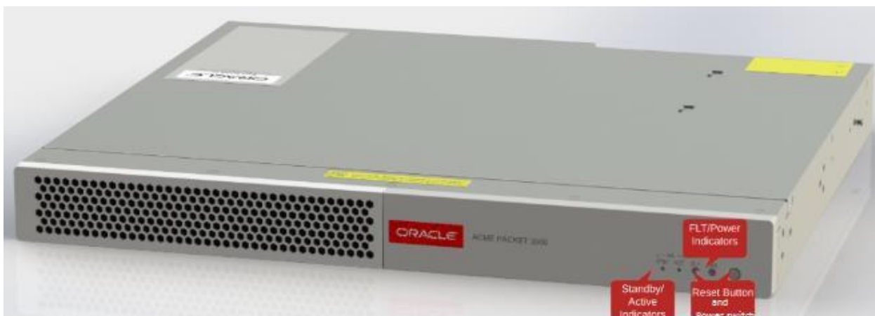
Figure 7: Acme Packet 3900 – Front View
