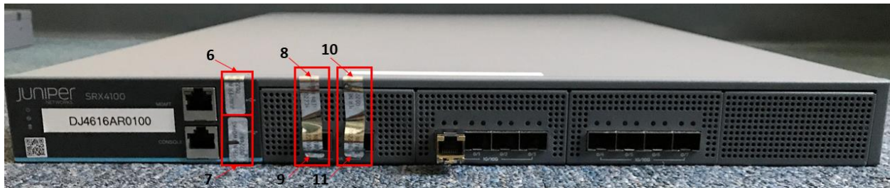
Figure 16 - SRX4100 & SRX4200 Front View: TEL 6-11
