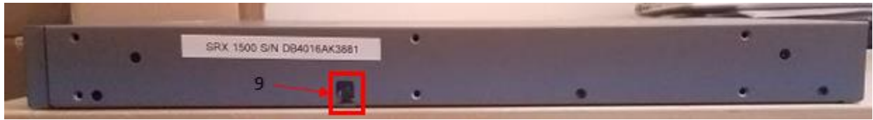
Figure 10 - SRX1500 Right Side View: TEL 9
