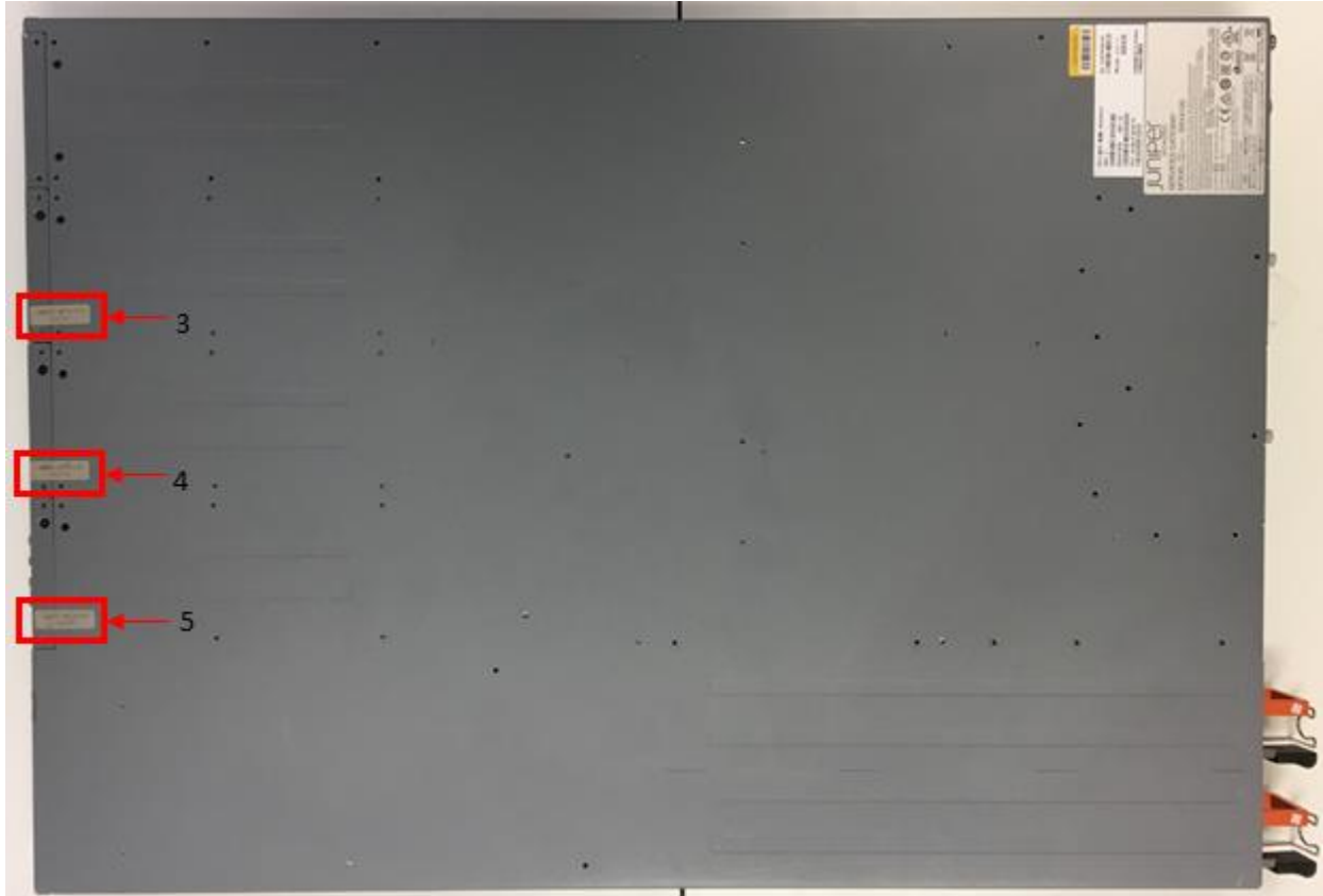
Figure 15 - SRX4100 & SRX4200 Bottom View: TEL 3, 4, 5
