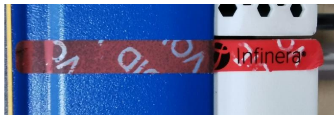
Figure 6 – Tamper-evident label: broken (close-up view)
