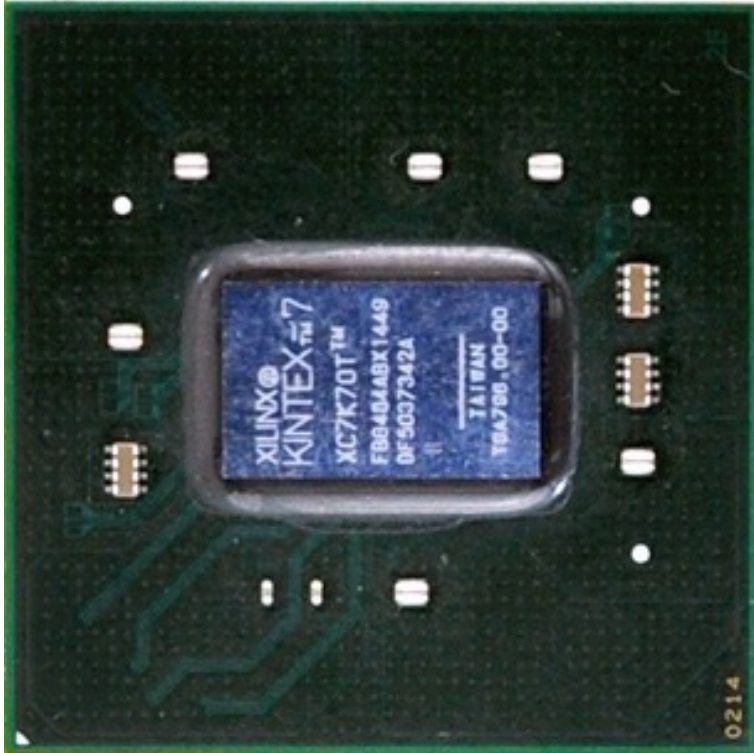
Xilinx Kintex 7 in flip-chip package
