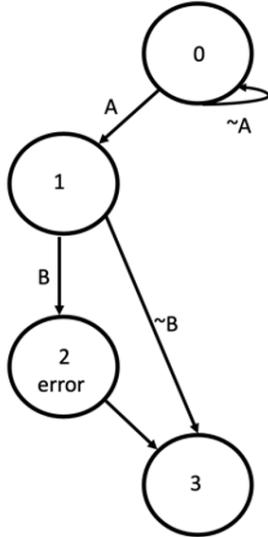
Fig. 5: Example Finite State Machine
