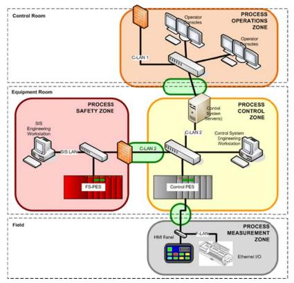
Figure 5 – Example of an Industrial Control System
