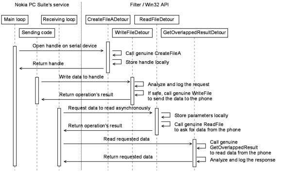
**Figure 7: Filter Sequence of Operations**
