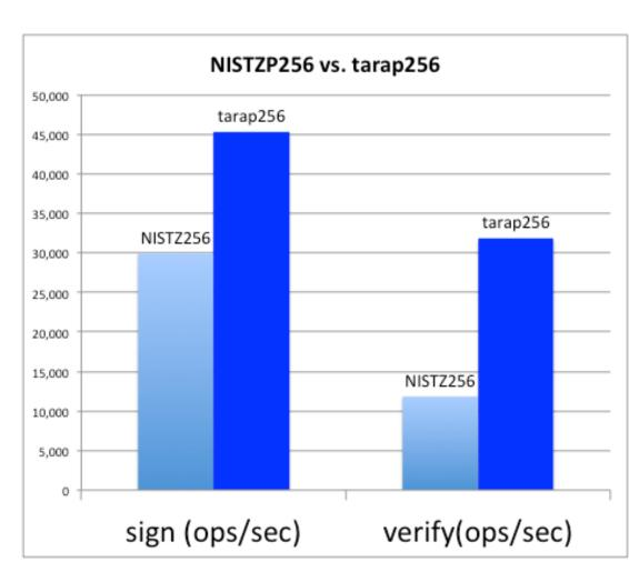
Measured on Intel® Xeon® E3 1275v3 Single core, Turbo & HT Off
