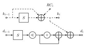
Fig. 2. Diagram of the critical of one unrolled AES round ( $RC_i$ : round constant,  $\ll$ : circular shift,  $\times$ : finite field multiplier). The dashed part is the key expansion, which does not impact the critical path.
