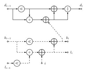
Fig. 8. Critical path diagram of one unrolled SPECK round ( $\ll$ : circular shift, i: round counter). The dashed part is the key expansion, which does not impact the critical path.
