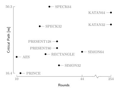
Fig. 9. Plot of the critical path on FPGA in function of the number of rounds.
