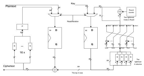
Figure 7. The datapath of the round-based RECTANGLE-80
