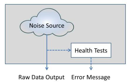
The continuous health tests monitor the noise source, and triggers an error message when it believes it detects a problem.
