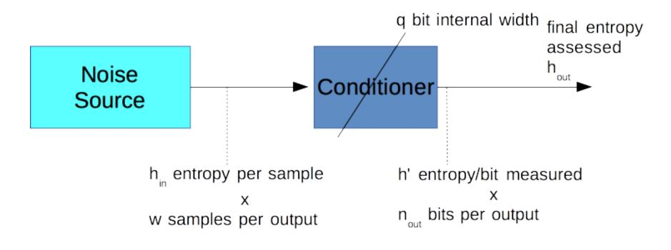
$h_{out} = \min(w \times h_{in}, 0.85n_{out}, 0.85q, h' \times n_{out}).$
