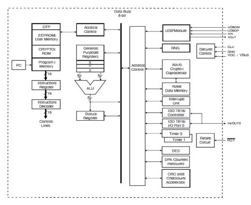
Figure 1: YpsID cryptographic module diagram
