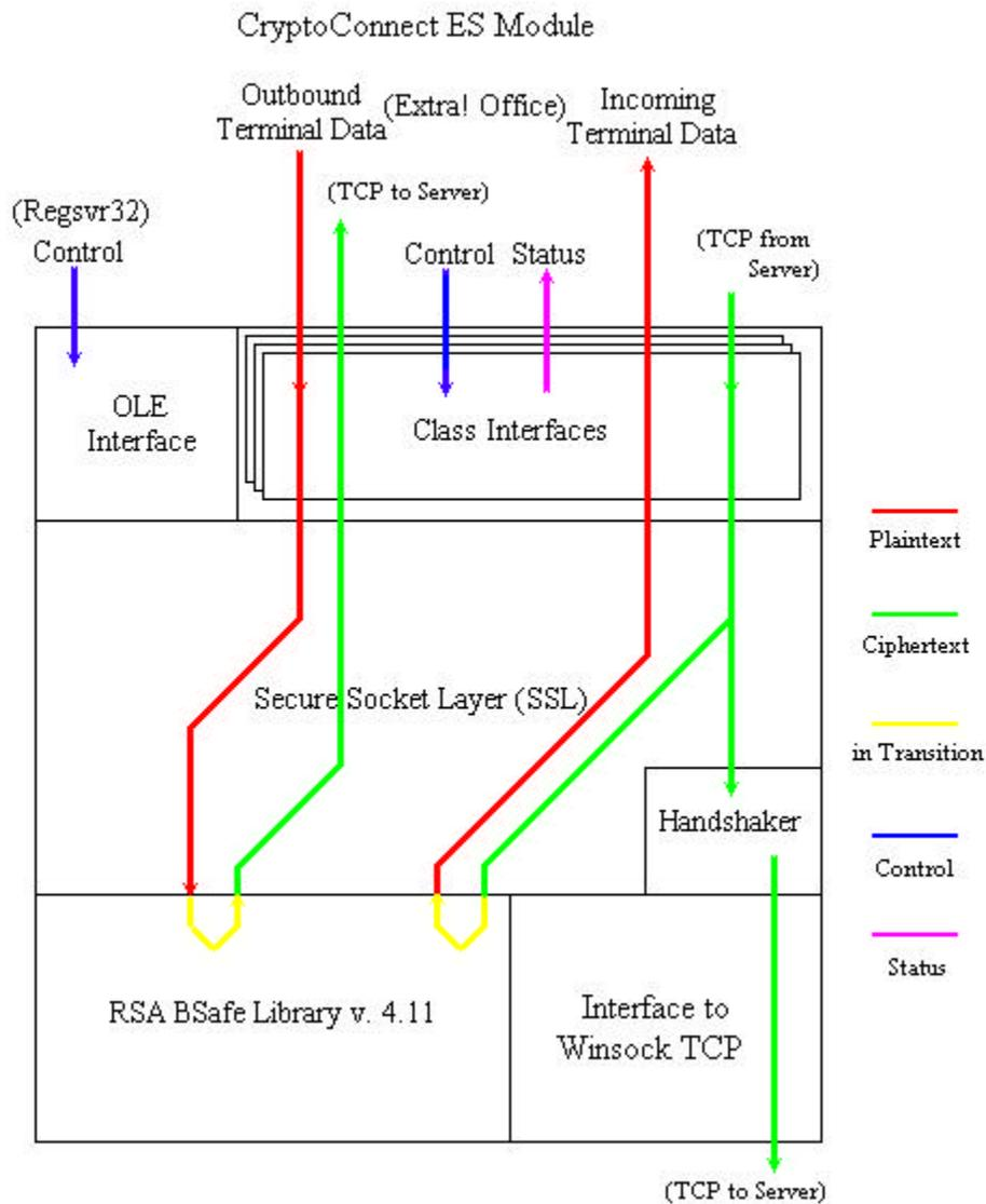
The **OLE Interface** contains control logic for access to the module.
