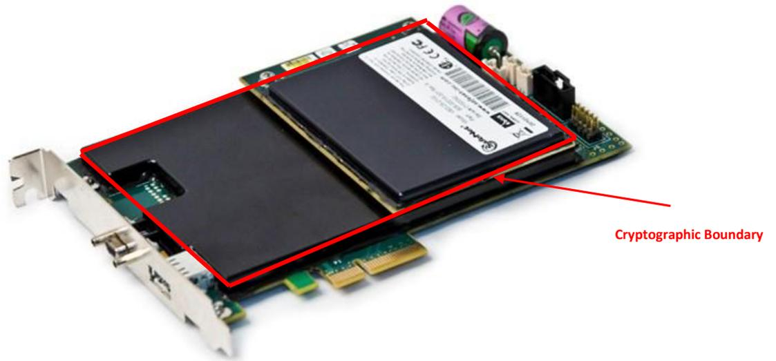
Figure 2-1. Luna PCI-E Cryptographic Module
