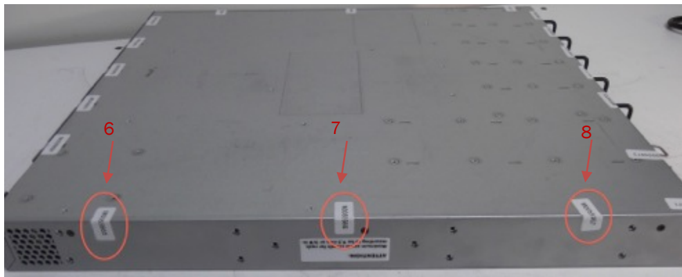
Figure 10 VDX 6740T-24, VDX 6740T-48, VDX 6740T-64 and VDX 6740T-56-1G bottom left side seal locations
