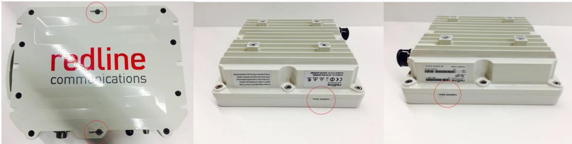
Figure 2 – Tamper-Evident Label Locations for RDL-3000 and Elte-MT
