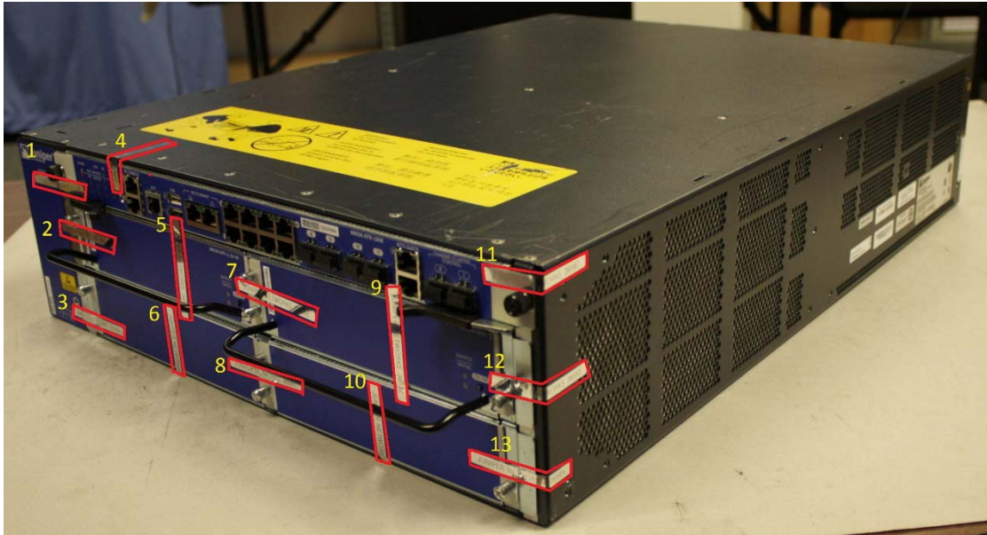
Figure 12: SRX3400 Tamper-Evident Seal Placement on Front and Right Side-13 Tamper Seals
