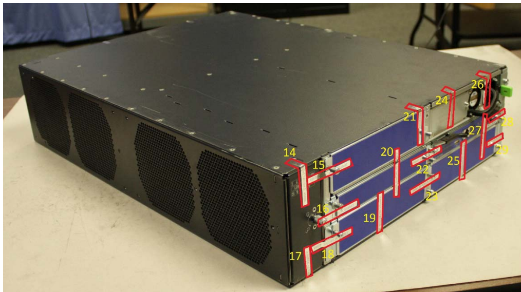
Figure 13: SRX3400 Tamper-Evident Seal Placement on Rear-16 Tamper Seals
