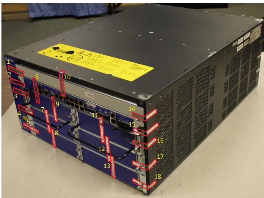
Figure 14: SRX3600 Tamper-Evident Seal Placement on Front and Right Side-18 Tamper Seals
