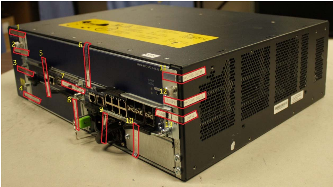
Figure 10: SRX1400 Tamper-Evident Seal Placement on Front & Right Side-13 Tamper Seals
