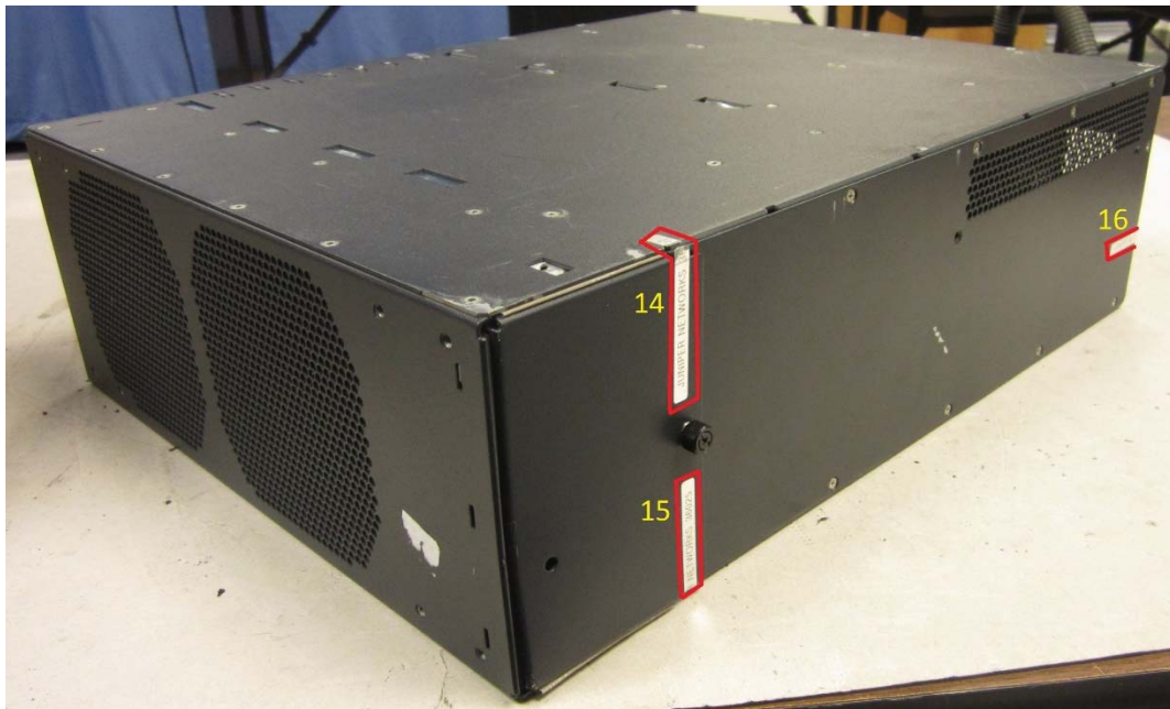
Figure 11: SRX1400 Tamper-Evident Seal Placement on Left Side-Three Tamper Seals
