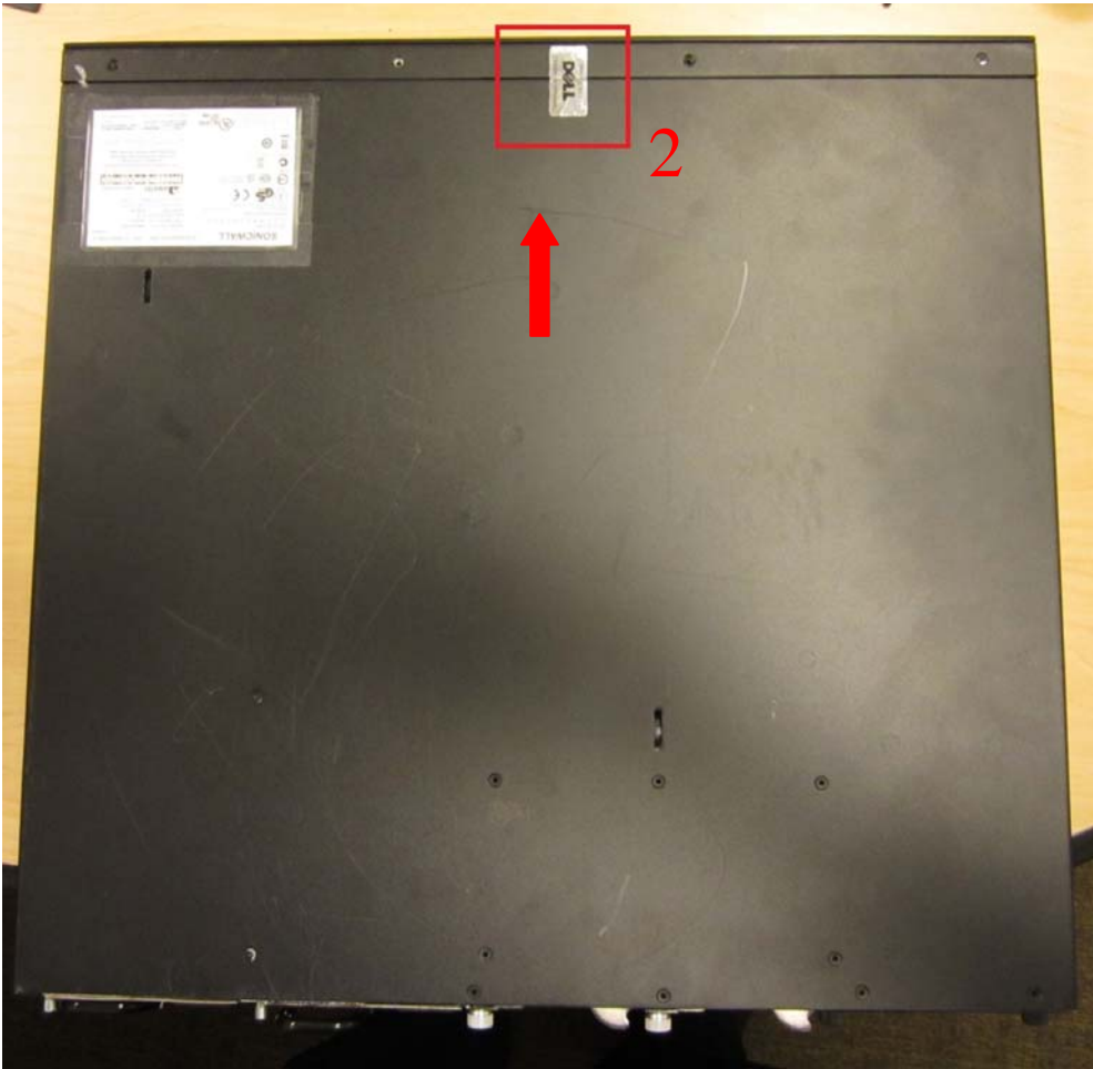
Figure 5 - SM Chassis with Tamper Seal Location on Underside, Front
