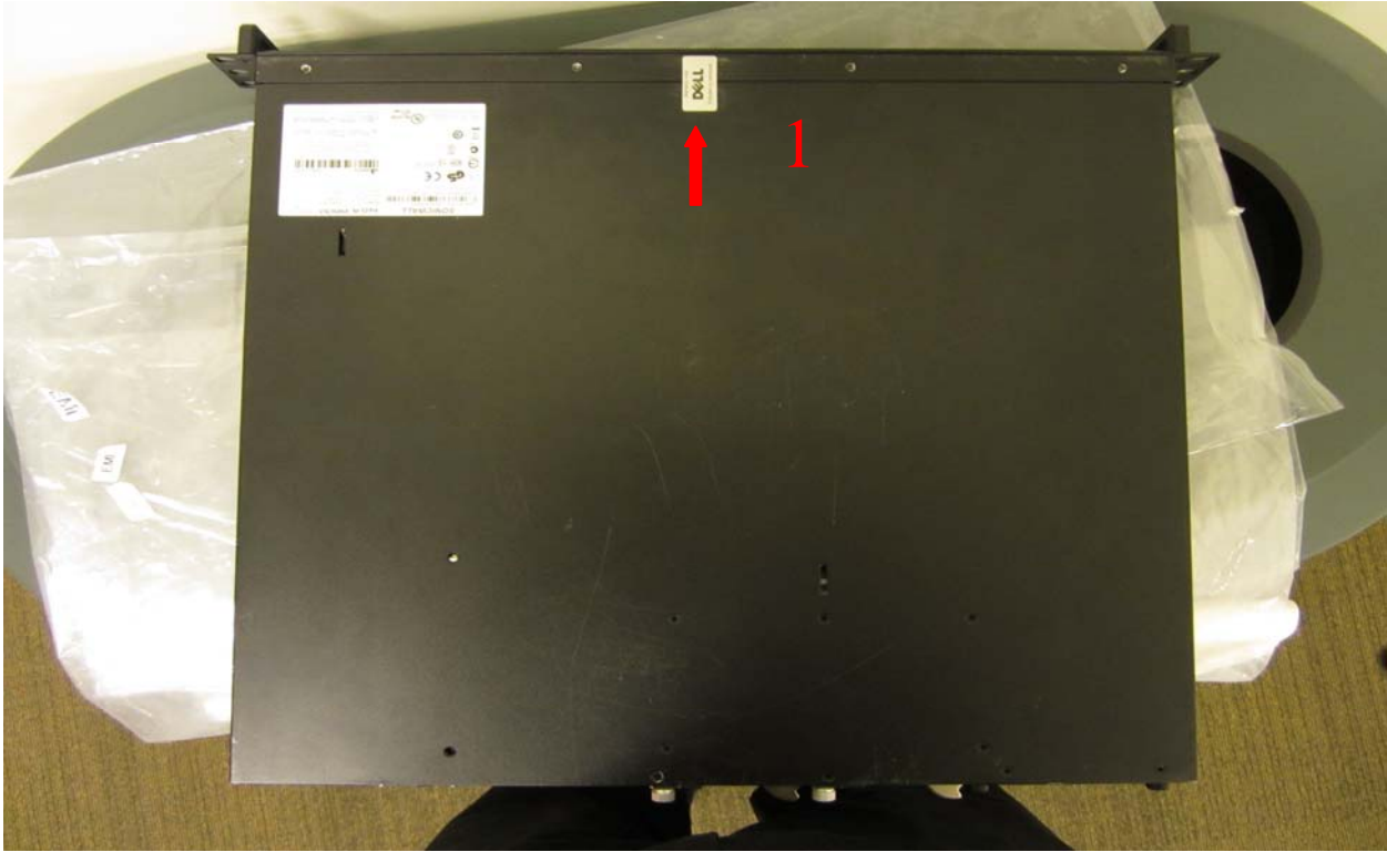
Figure 2 - NSA 6600 Tamper Seal Location on Underside, Front
