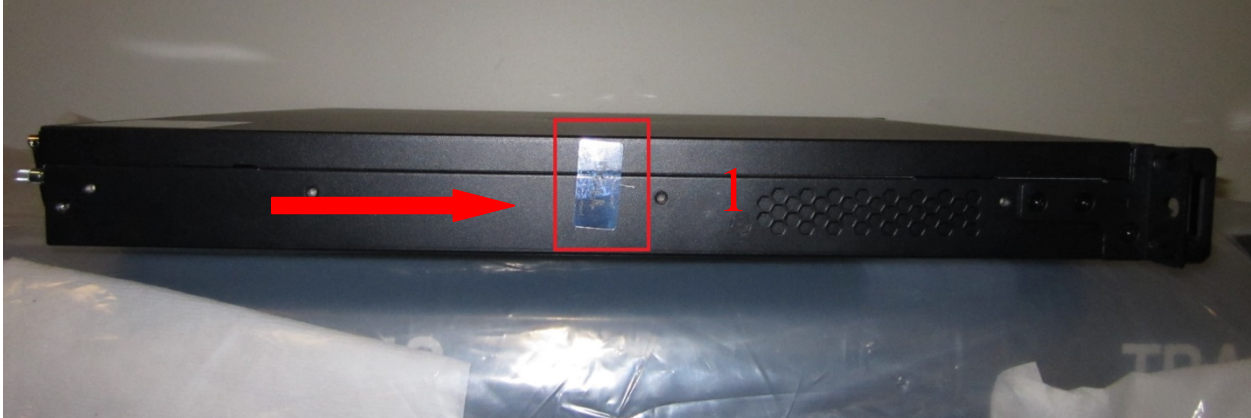
Figure 4 – SM Chassis with Tamper-Evident Seal Location on Left Side
