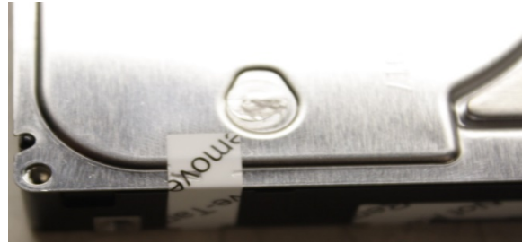
Figure 4: Tamper Evidence on Large Tamper Label Figure 5: Tamper Evidence on Metal Surface
