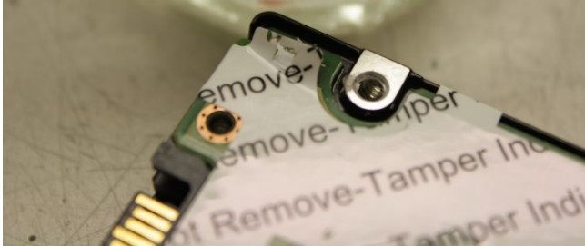
Figure 4: Tamper Evidence on Large Tamper Label Figure 5: Tamper Evidence on Metal Surface
