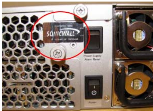
Figure 7 – SRA EX9000 Tamper Seal #5 - Rear Fans
