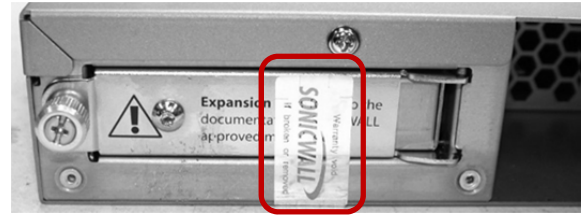
Figure 4 – Tamper Seal #3 – Expansion Bay
