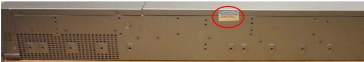
Figure 5 – SRA EX9000 Tamper Seal #1 - Right Side
