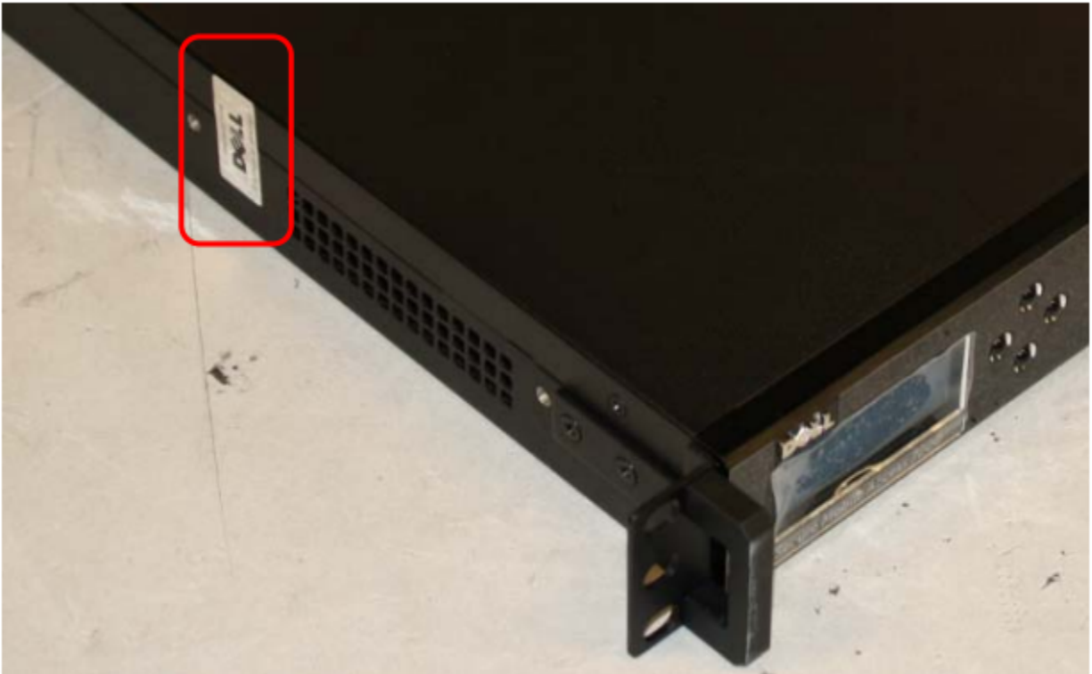
Figure 9 - SMA 6200 / SMA 7200 Tamper Seal #1 - Chassis Seam
