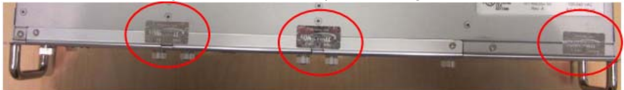
Figure 6 –SRA EX9000 Underside Tamper Seals #2, #3 and #4
