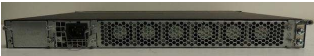
Figure 11 - BR-CES-2024C-4X-AC backside with Power supply: RPS9 (AC Power supply)
