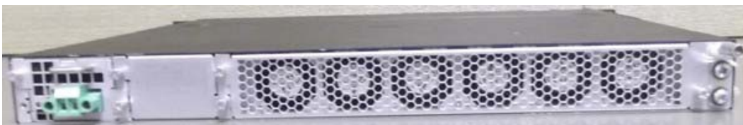
Figure 5 - BR-CER-2024C-4X-RT-DC backside with Power supply RPS9DC (DC Power Supply)
