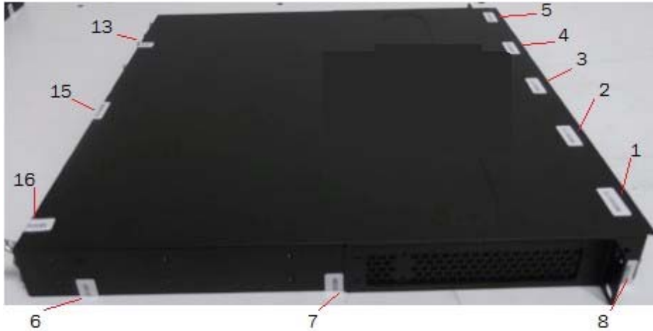
Figure 20 - Left side view of Brocade CER 2024C-4X-RT device with security seals
