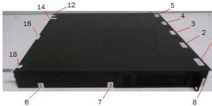
Figure 35 - Left side view of Brocade CES 2024F-4X device with security seals
