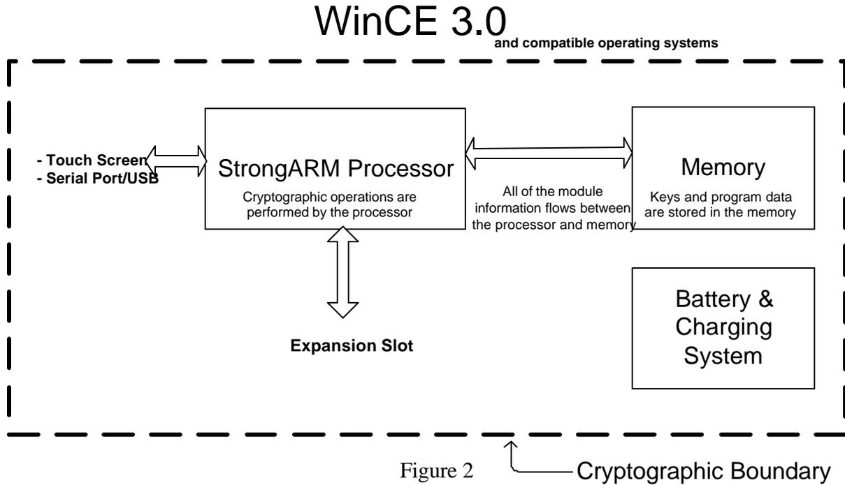
Figure 2 Cryptographic Boundary
