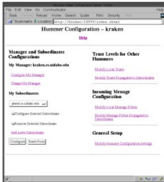
Figure 3: Main Configuration Window for Individual Hummer: set peers, managers, subordinates; assign behavior for handling alerts and alarm situations; handle data filtering; etc
