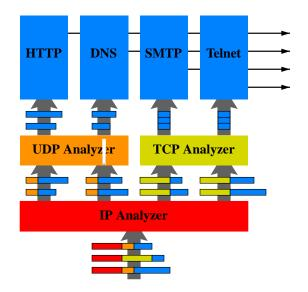
Figure 2: General schematic for a network monitor stack, including suggestions of the kinds of information available at different levels.
