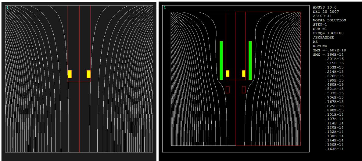
Fig. 8 Effect at sensor (yellow) of magnetic shield (green) on field by noise source at large distance (outside figure)
