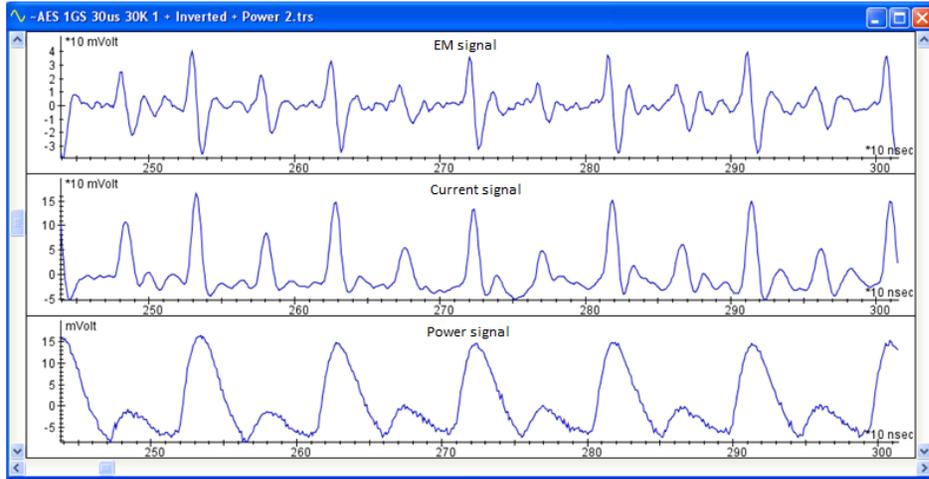
Fig. 5 From top to bottom the EM probe signal, the current signal and the simultaneously measured power consumption
