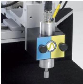
Fig. 19 Riscure HS probe with XYZ stage and magnetic shield.
