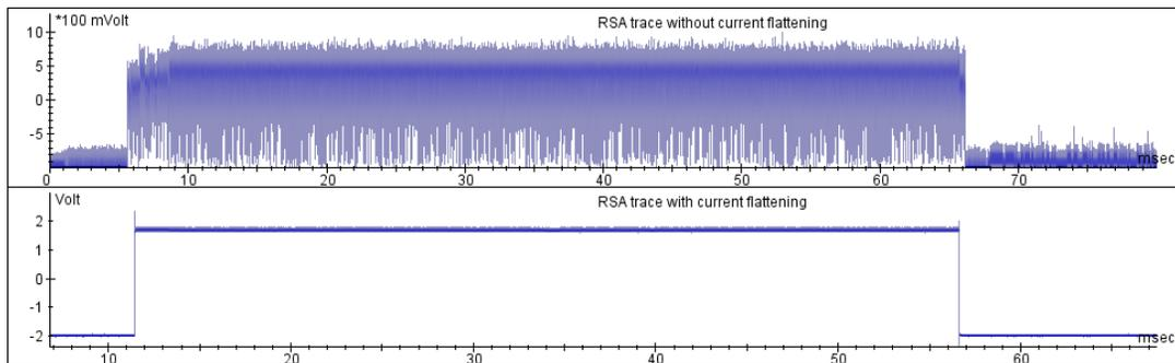
Fig. 3 Power signal without and with current flattening
