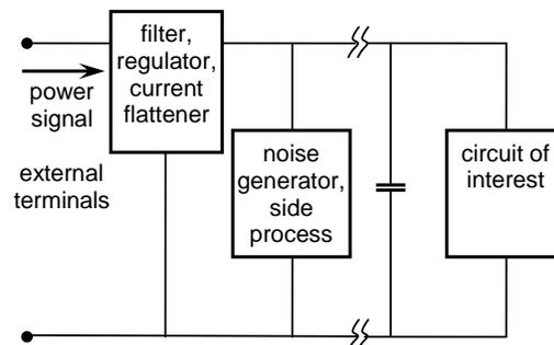
Fig. 2 Simplified chip circuit diagram, showing connections between terminals, filter, noise generator and circuit of interest.
