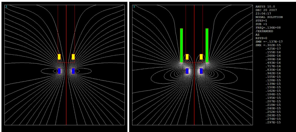
Fig. 9 Effect at sensor (yellow) of magnetic shield (green) on field by noise source (blue) close to shield aperture
