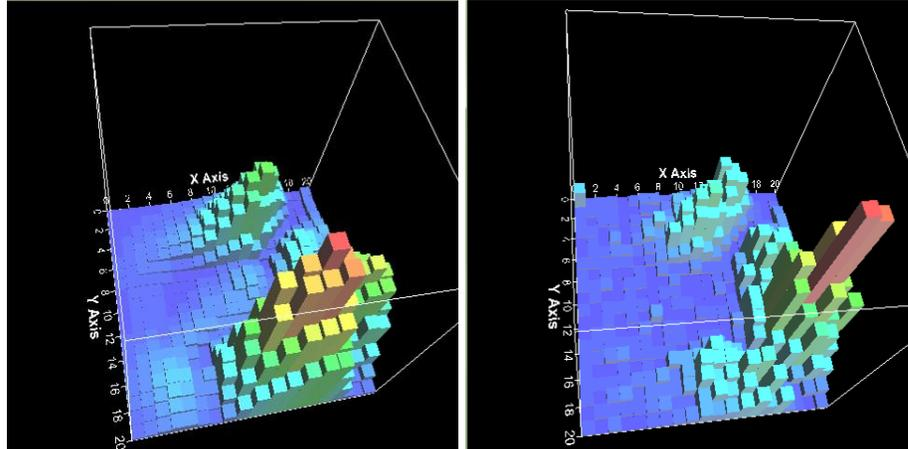
Fig. 11 Illustration of 2x2 mm XY scan over smart card surface: left for external clock frequency, right for internal clock frequency.
