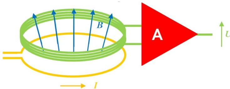
Fig. 4 Orientation of current loop (yellow) and sensor coil (green)
