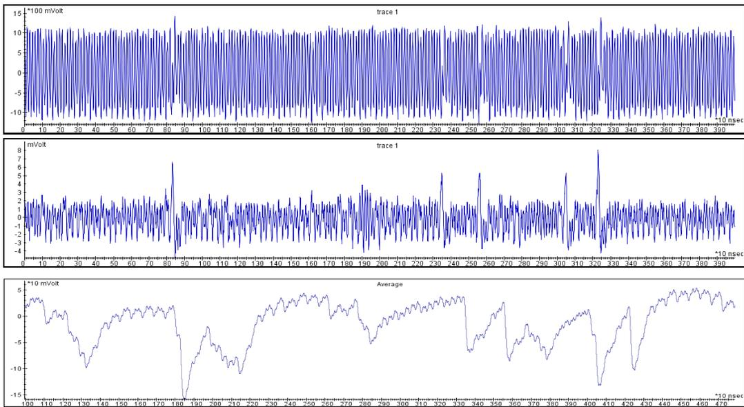
Fig. 23 From top to bottom: signal from B-, H- and current probe with 90 MHz low pass filter
