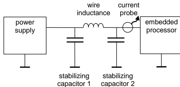
Fig. 1 Simplified connection scheme between power supply and embedded processor.
