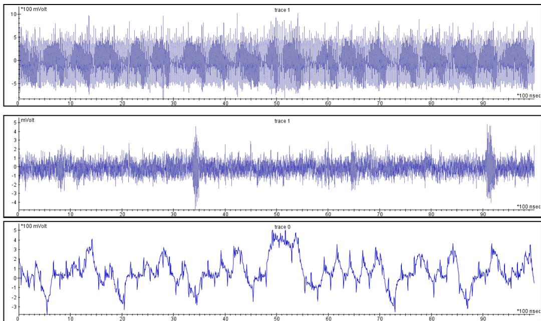
Fig. 25 From top to bottom: signal from B-, H- and current probe with 90 MHz low pass filter
