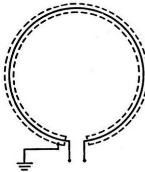
Fig. 6 Electrical shield of single winding coil.
