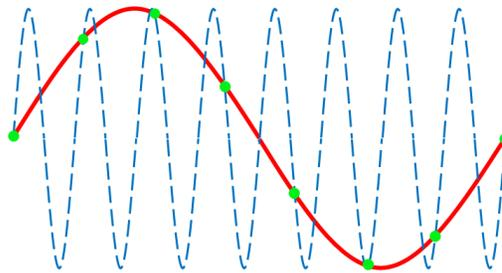
Fig. 10 Illustration of aliasing: the reconstructed signal through the sample point of the analog input signal (dashed line)
