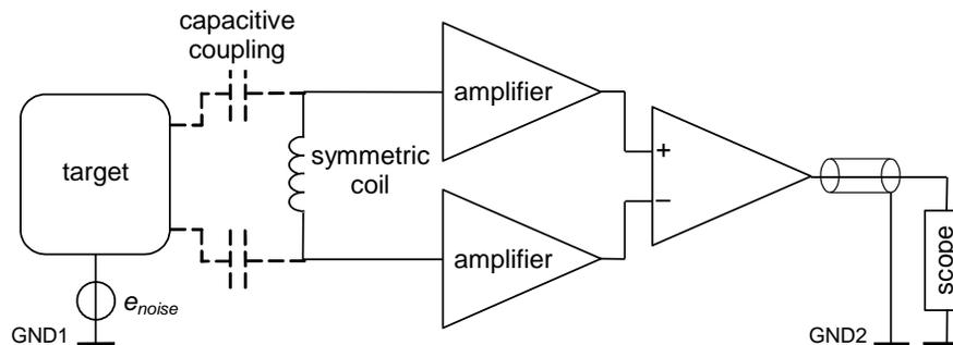
Fig. 7 Differential amplifier with symmetric coil.
