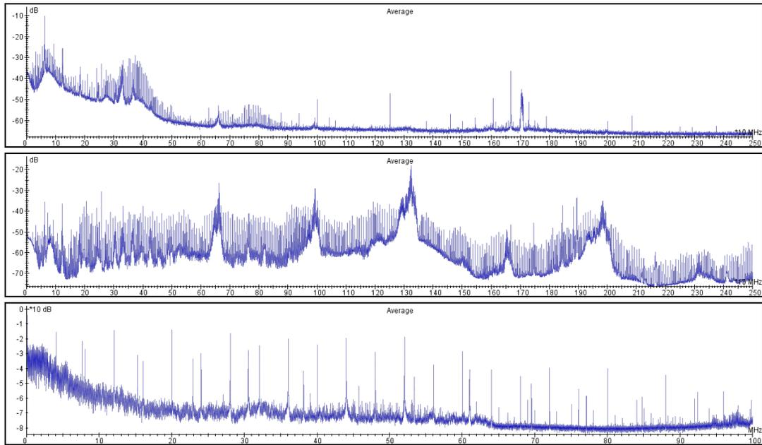
Fig. 24 From top to bottom: spectra of B-probe, H-probe and current probe (different frequency scale)
