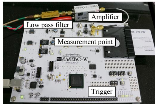
**Figure 9:** Measurement environment for power trace.
