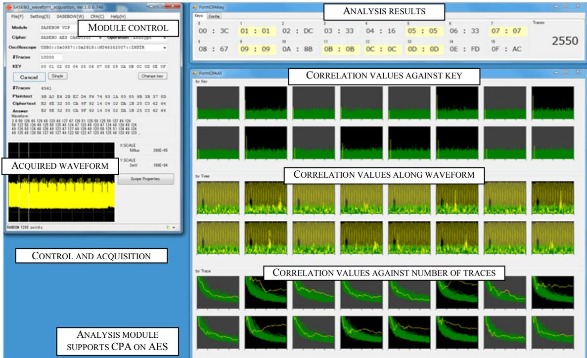
FIGURE 4: Side-channel attack evaluation software.
