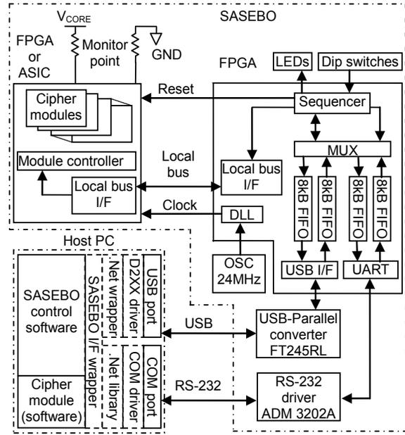
Figure 3: Block diagram of control HW/SW on SASEBO.
