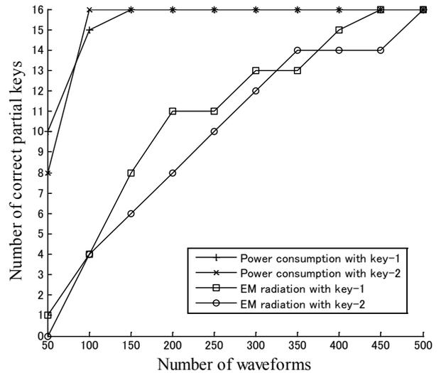
Figure 13: Number of correct partial keys versus number of power trace waveforms.
