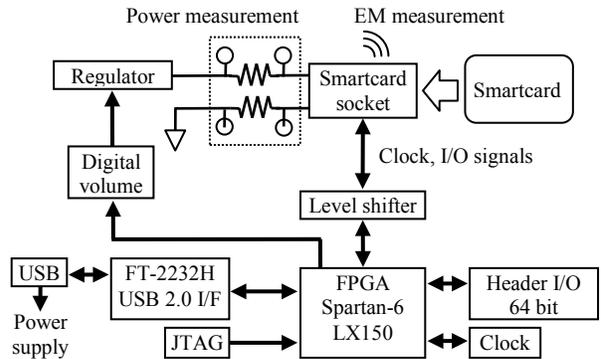
Figure 6: Block diagram of SASEBO-W.
