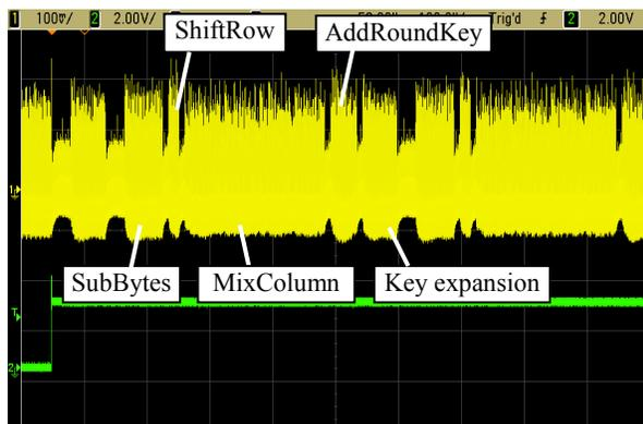
Figure 12: Magnified view of the power consumption waveform.
