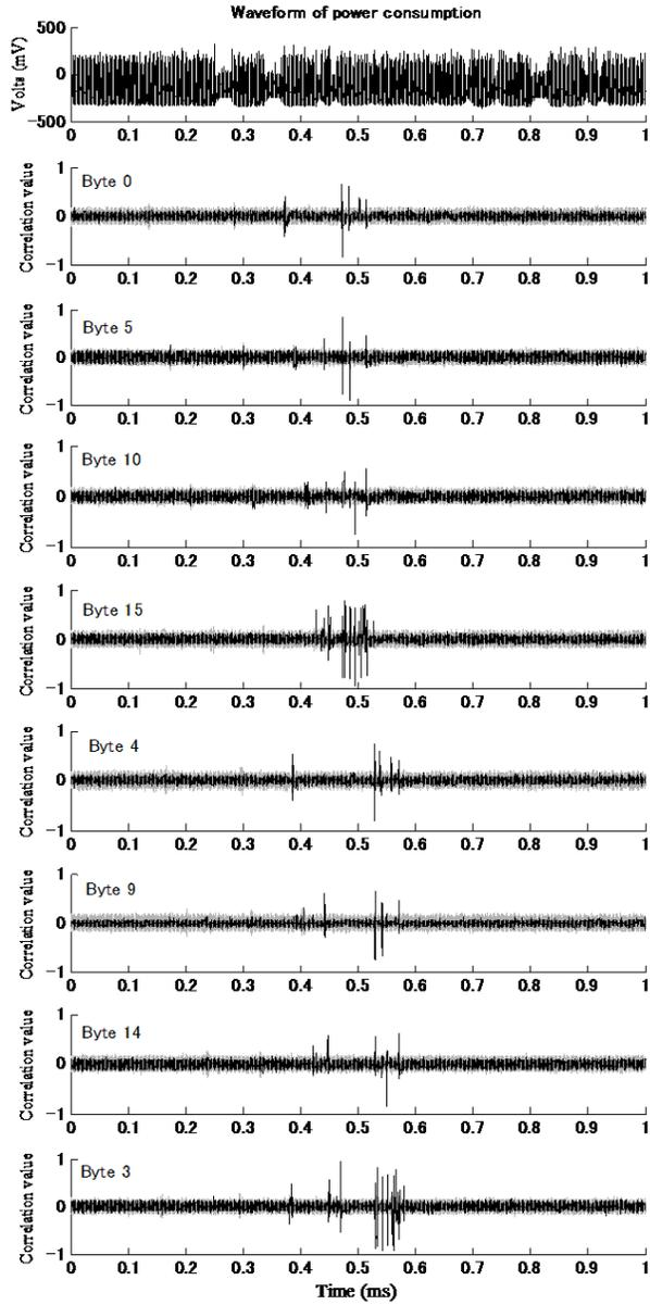
Figure 20: Correlation values plotted against time in matching the peaks to the MixColumn function.
