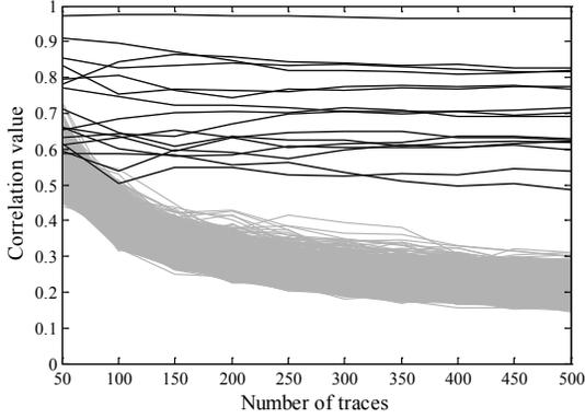
Figure 15: Correlation values of power waveforms with key-2.
