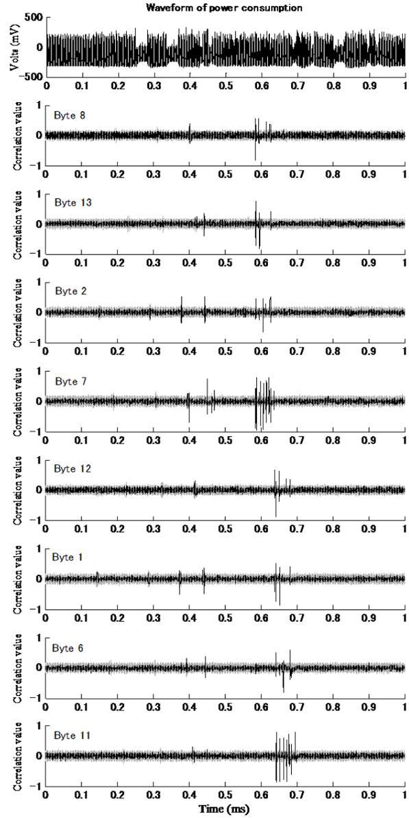
Figure 21: Correlation values plotted against time in matching the peaks to the MixColumn function.
