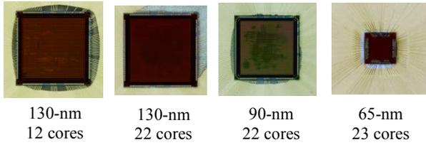
Figure 2: Cryptographic LSIs.
