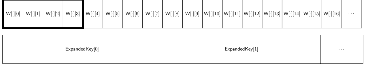
Figure 1.7: Key expansion and round key selection for N_b = 8 and N_k = 4 .
