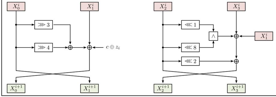
**Figure 3:** Round function of SimP, which is equivalent to SIMON-2w/2w with its key schedule, where  $w$  is the word size. It transforms the four-word state  $(X_0^{i-1}, X_1^{i-1}, X_2^{i-1}, X_3^{i-1})$  to  $(X_0^i, X_1^i, X_2^i, X_3^i)$ .
