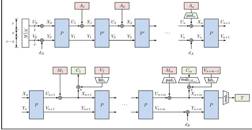
**Figure 1:** Schematic illustration of the authentication of an  $a$ -block associated data  $A$  and the encryption of an  $m$ -block plaintext  $M$  with Oribatida, for  $m > 1$ .  $P$  and  $P'$  are permutations,  $K$  the secret key,  $N$  the nonce,  $C$  the resulting ciphertext, and  $T$  the resulting authentication tag.
